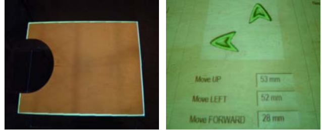
Figure 2: Left: a bright rectangle formed by the 4 bright blobs. Right: real time visual feedback projected on the table. The arrows indicate where to move the table. The texts indicate how much to move. For example: Move FORWARD 28mm, as shown at the bottom in the right figure.
