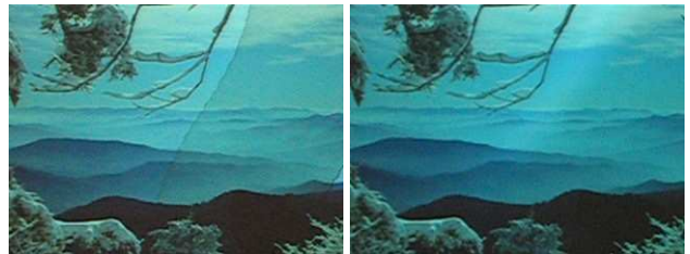
Figure 3: Boundary between regions of varying projector ownership. Left: before seam blending Right: after seam blending
