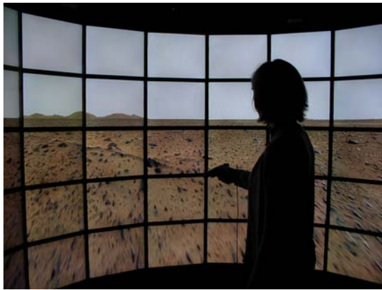
Figure 1: The Varrier display has 35 panels mounted in a semi-circular arrangement to provide wide angles of view in an immersive VR environment.
