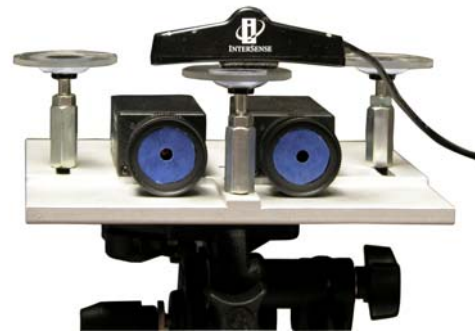
Figure 3: Two parallel video cameras separated by interocular distance simulating human eyes.
